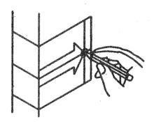
Start approximately 38" (965mm) from floor. Fold and apply template to high edge of door bevel and mark center hole on door face through guide on template for 2-3/8"(60mm) or 2-3/4"(70mm) backset.
