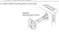
b. Press inside rose liner onto mounting plate and tighten mounting screws securely.
