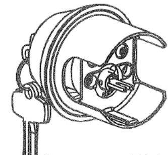
Load the tailpiece in the vertical direction and turn 90 degrees to horizontal position.
