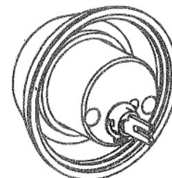
Load the tailpiece in the horizontal direction and turn 90 degrees to vertical position.
