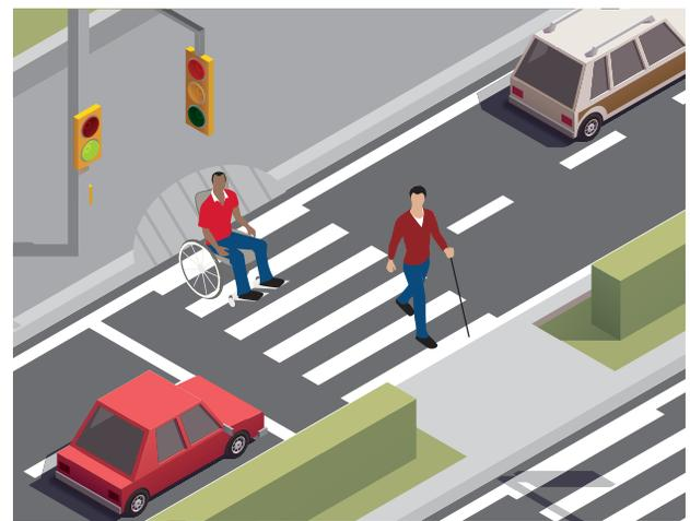
37. A 1,500 mm x 1,500 mm level surface shall be maintained on the sidewalk behind the curb ramps.
