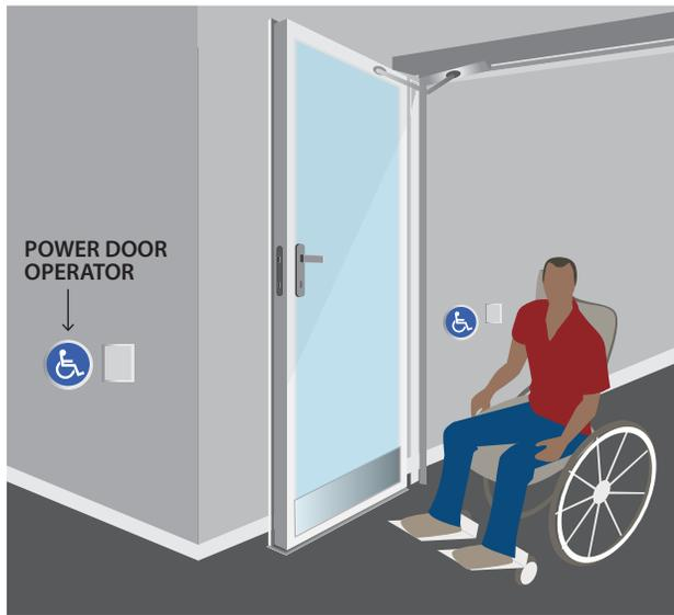
72. If an entrance has a power door operator, and there is a vestibule immediately inside the doors, the vestibule doors shall also be equipped with a power door operator.
