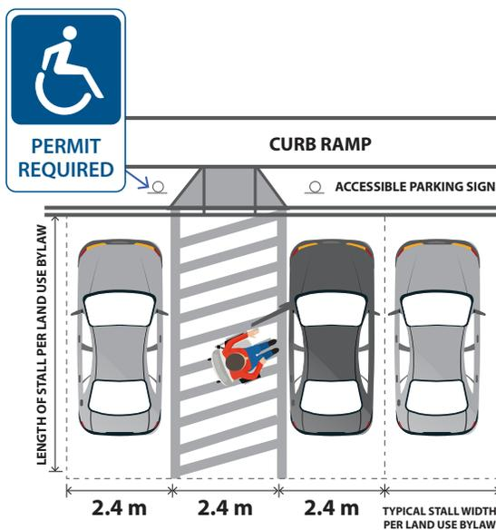
4. Parking stalls shall be designed so that vehicle bumpers or other obstructions do not encroach on the barrier-free path of travel, regardless of the width of the path of travel.
