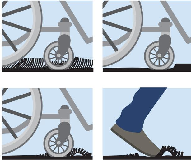
90. All floor surfaces shall be slip-resistant, non-glossy and stable. The co-efficient of friction shall be no less than 0.5 when wet or dry.
