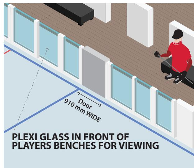
221. The player's bench areas shall be designed to have removable benches or shall have a minimum of 900 mm between the bench and surrounding boards or walls.
