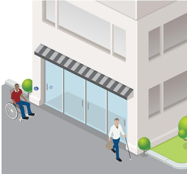
Explanation: If an entrance has three doors, there shall be one set of double doors and the third door can be hinged on either the left- or right-hand side. As another example, if there are two doors in a series, the inner door and outer door should be hinged on opposite sides.
