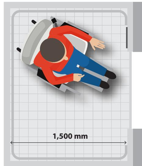
**THERE SHALL BE ENOUGH SPACE IN AN ELEVATOR CAR TO ALLOW A PERSON IN A WHEELCHAIR TO TURN AROUND**
