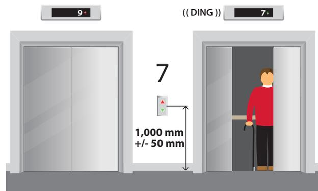
**AN AUDIBLE SIGNAL SHALL INDICATE WHEN THE CAR HAS STOPPED AT EACH FLOOR**
