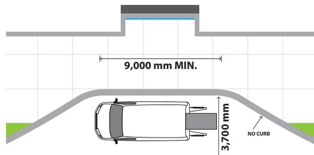
15. Where Calgary Transit Access or Calgary Transit vehicles stop near a building entrance, at least one passenger loading zone shall be designed in accordance with the Alberta Building Code 2014 3.8.2.2.(3), Calgary Transit requirements and these standards.
