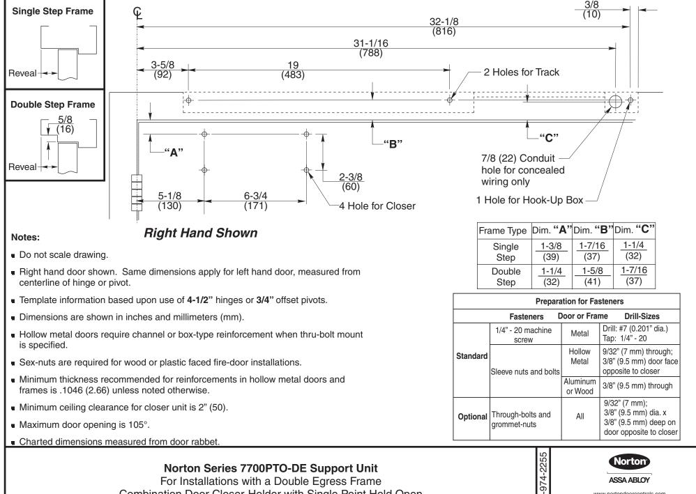
Combination Door Closer-Holder with Single Point Hold Open Hinge (Pull) Side of Door Installation with Hinge Side Frame Reveals 1/8" to 3" (3 to 76mm)
