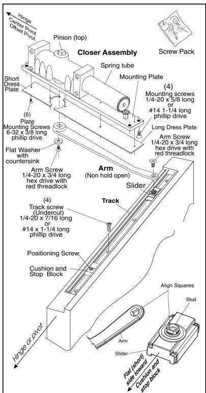
• Set door opening angle. Open door to the angle you want the door to stop. With the door held at that location, slide cushion and stop block against slider. Tighten the stop position screw (large set screw) with 3/16" hex wrench (from screw pack) until secure. Release door.
