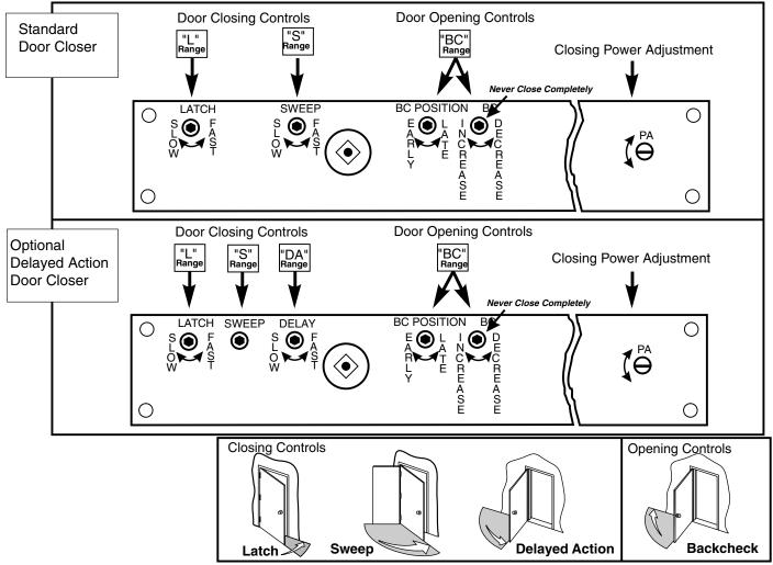
Closer Controls accessible through mounting plate for closer adustment: Use 1/8" (3mm.) hex-key for valve adjustments.
