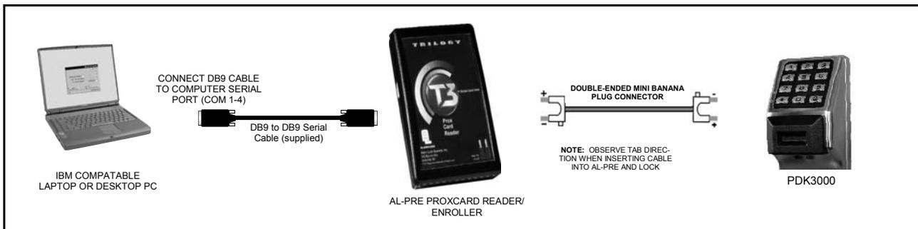
**Scenario 3** Enroll ProxCards® quickly into DL-Windows, then transfer this new ProxCard® data from the computer through the AL-PRE to the lock (thus avoiding the need to use an AL-PCI cable). For PDK series locks only.
