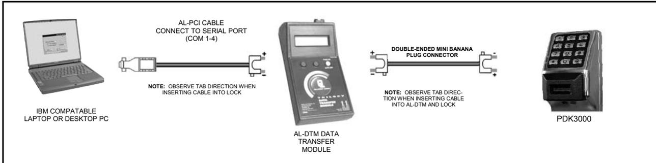
**Scenario 2** Create the program in DL-Windows and transfer the program from your computer to an AL-DTM (via an AL-PCI cable)... then transfer the program from the AL-DTM to the lock(s) (via a double-ended mini banana plug). The hand-held AL-DTM is useful because you do not have to transport (or find electricity for) your computer. Data can also flow in reverse, from the lock, through the AL-DTM, back to the computer for examination.
