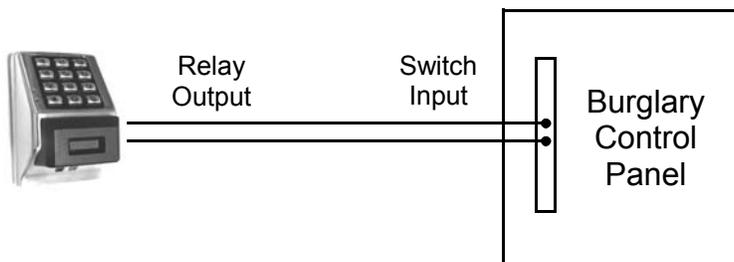
Alarm Panel with Switched Input for Disarming
