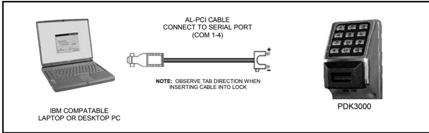
If your computer does not have a serial COM port (DB-9 male) available, you can plug your AL-PCI cable into a special USB to RS-232 cable. Order part PCI-USB for the USB to RS-232 cable only, or ALPCI2-U for both the USB to RS-232 cable and an AL-PCI2 cable).
