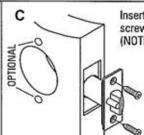
Insert latch and tighten screws.
