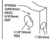
Drill 2-1/8" (54mm) hole through door face and two holes 13/64" (5mm),Drill 1" (25.4 mm) hole in center of door edge for latch. OPTIONAL:
